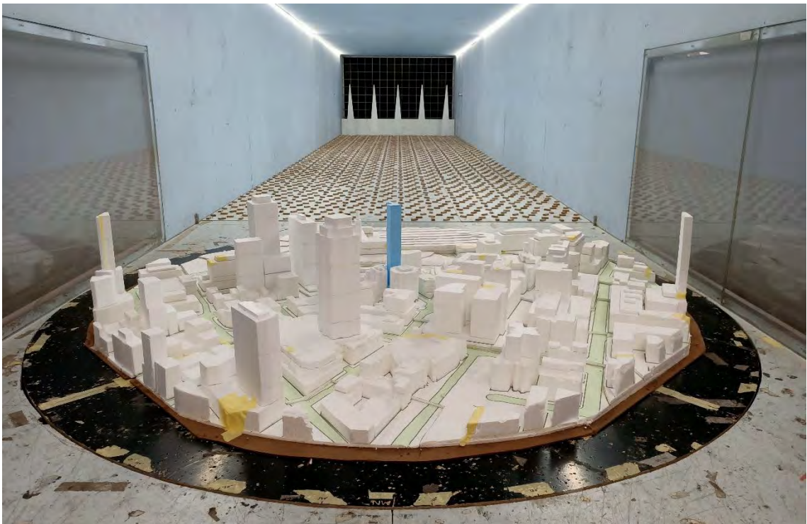
Figure 1c: Photograph of the Wind Tunnel Model (Base Case, view from the north-west)
